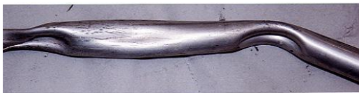
Above and below, outboard end of centre push rod illustrating crushing and arcing damage at outer end only.
