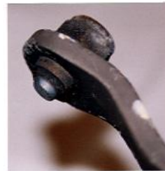
Airbrake mechanism, sooted but unaffected Aileron system bellcrank (distorted) Fuselage side rib Cracked push rod apertures Fuselage side rib Controls in fuselage centre section, illustrating extent of sooting
