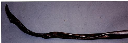
Above and below, outboard end of centre push rod illustrating crushing and arcing damage at outer end only.
