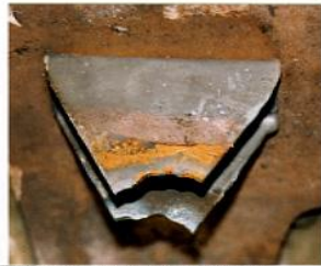
Right aileron bellcrank mounting bracket showing melted end and heat effects
