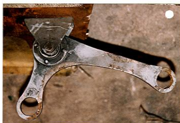
Left aileron bellcrank, found attached to support bracket and section of spar. Attachment bolts were undamaged.
