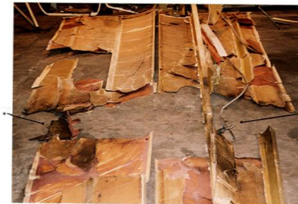
Detail of left wing structure in region of aileron actuator rod/bellcrank*
